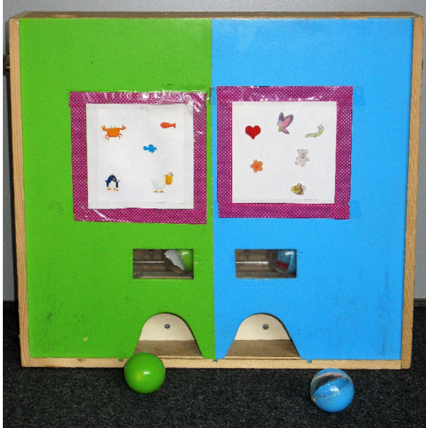
Fig. 1. Sticker dispenser with blue and green sides containing half-transparent plastic balls with two different kinds of stickers. A marble needs to be inserted into one of two holes on top of the apparatus to release a ball of the corresponding color. (For interpretation of the references to color in this figure legend, the reader is referred to the Web version of this article.)
