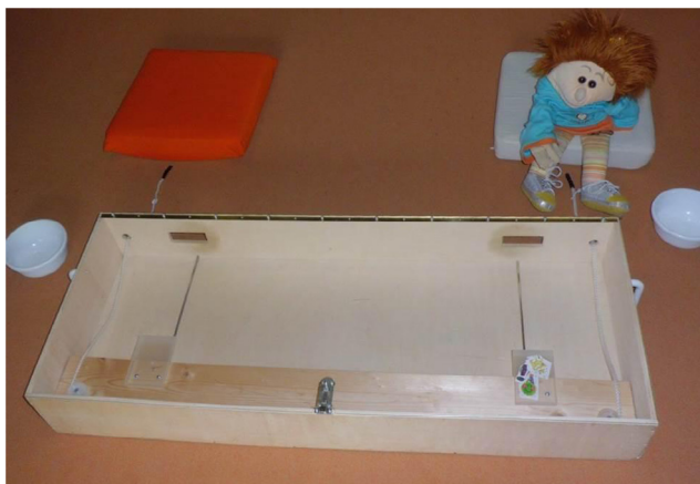
Fig. 1. The setup used in Study 1. The child sat on the pillow next to the puppet (here: the empty pillow). The box was covered with Plexiglas, and the child and puppet needed to pull the rope together to move the board with the stickers toward them. The stickers could then be retrieved through the hole in front of the puppet and the child, respectively.
