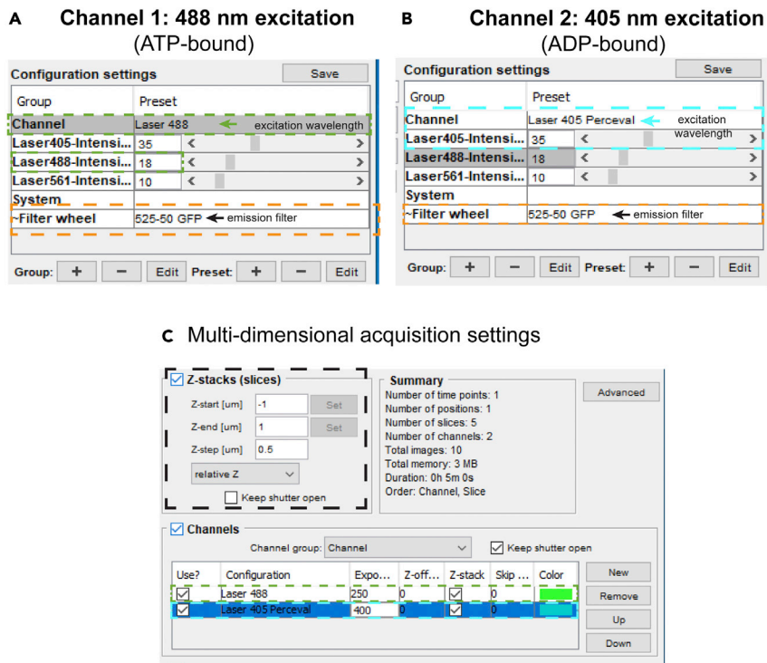
Figure 3. Microscopy settings for Zeiss AxioImager A1 (spinning-disk confocal) in Micromanager, related to step 6 (A and B) This figure displays the two acquisition channels for PercevalHR image acquisition. The excitation wavelength and laser power settings for the ATP-bound state are highlighted in green-dashed boxes (Channel Laser 488) and the excitation wavelength and laser powersettings for the ADP-bound state are highlighted in cyan-dashed boxes (Channel Laser 405 Perceval). The emission filter wheel wavelengths highlighted in orange-dashed boxes. (C) Optimal settings for z-stack acquisition of PercevalHR images. The black-dashed box highlights the start and end positions and z-step size of the intended z-stack (in µm). The green and cyan-dashed boxes highlight the exposure timing (in ms) of the ATP-bound (Channel: Laser 488) and ADP-bound (Channel: Laser 405 Perceval) respectively.
