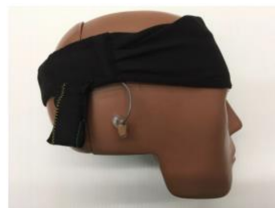
Fig. 2. The Data Acquisition System for Head Response (DASHR) earpiece on a dummy head.
