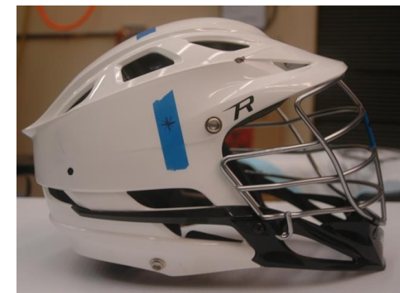
Fig. 1. Parietal right impact location (as indicated by the crosshair) on the lacrosse helmet in which the head was placed.
