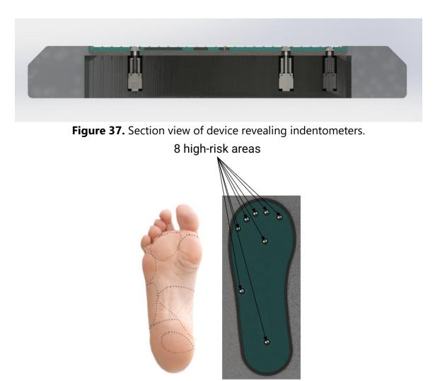
Figure 38. Indentometers located in high risk areas of the plantar surface.
