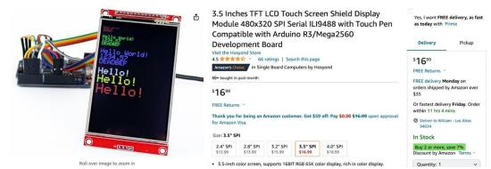
Despite indicating that it is Arduino compatible, the ILI9488 requires a GPIO logic level of 3.3 V. As such, we also plan to purchased logic level converters, which are SPI compatible
