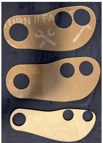
Figure 4. Laser Cut Acrylic/Wood Foot Cutouts
