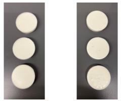
*Non-Callused (1.2 MPa) Callused (2.3 MPa)* **Figure 80.** Alginate Samples with Different Moduli.
