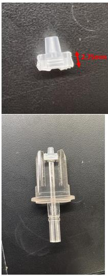
Then drill out the hole with the ~2.1mm drill bit in the 11044 bin. This widens the part and makes a tighter seal in the OneDraw. Ideally, there will be a ~2mm gap between the bottom of the female gray part and the flat face of the PP tapered part. You can feel the snug fit when inserting the part.
