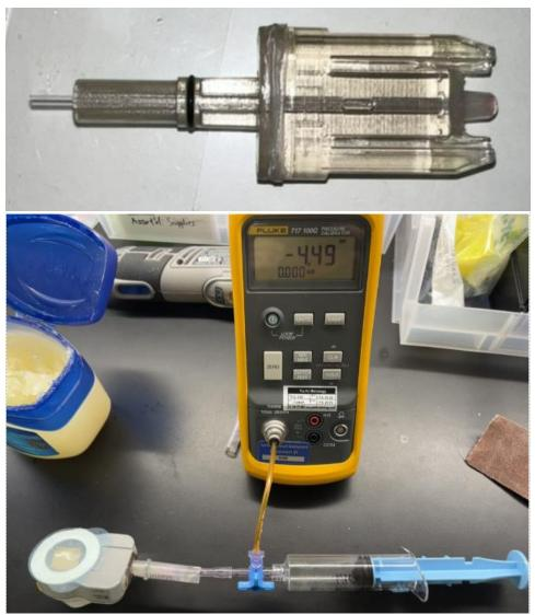
5. Record the mass of the vial. Reapply Vaseline to the adapter o-ring and then slide the vial on and record the mass of the whole device (including plastic cover and vial, but not including the PSA). When calculating the volume collected, assume a density of 1 g/mL and calculate both the total volume collected by the device (which includes blood left inside the capillary and the cup) and the volume collected just by the vial.
