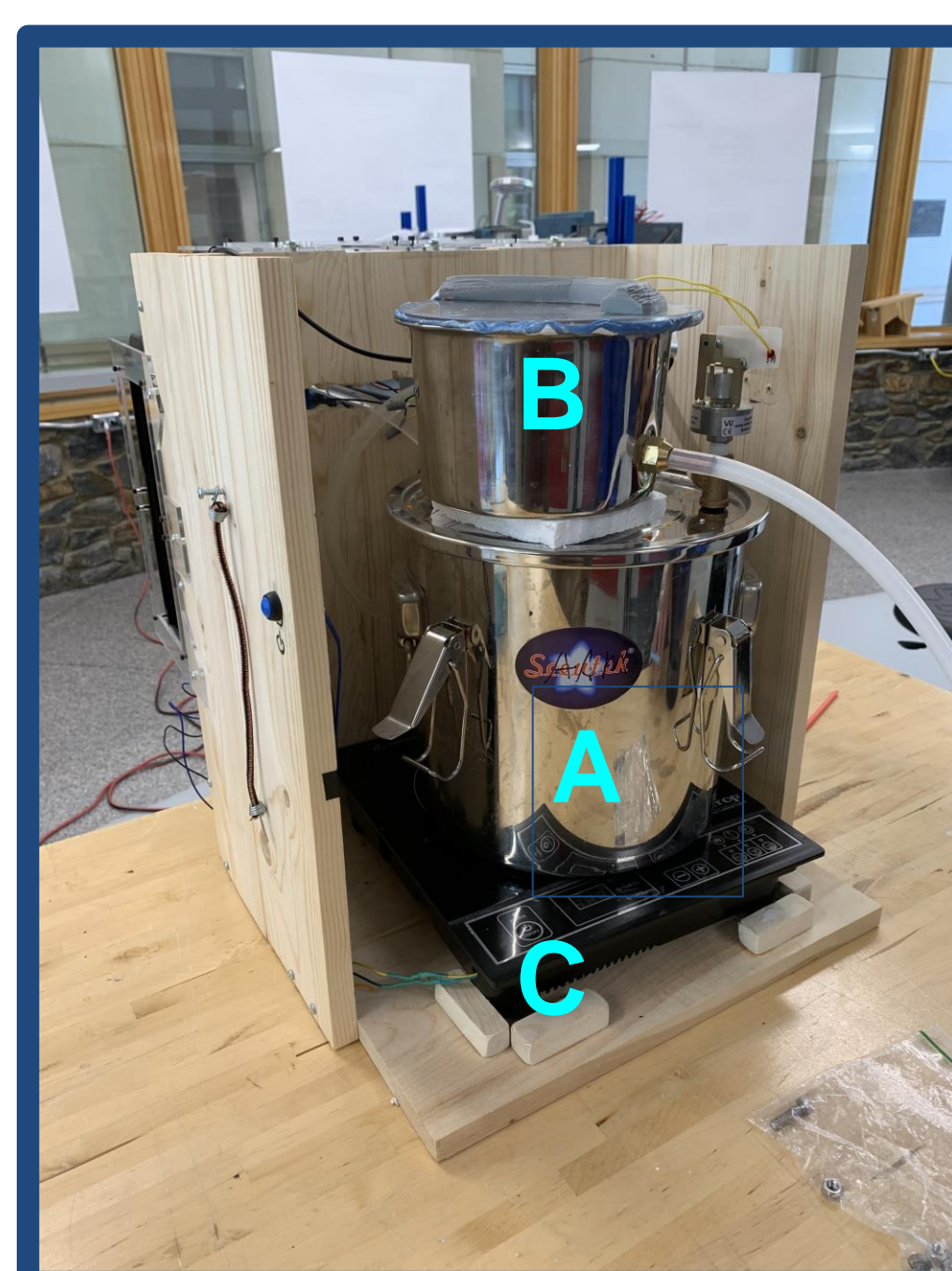
Final automated prototype – singular press of the power button initiates distillation cycle
