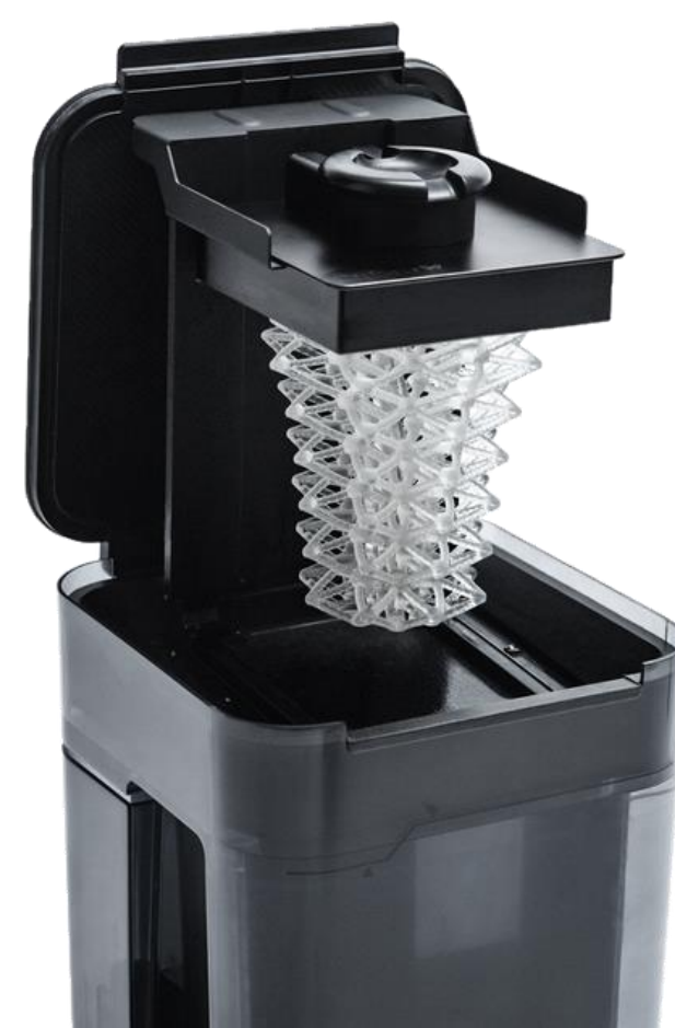
A FormLabs wash station used to clean prints with IPA
