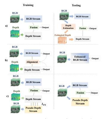
Figure 1: Comparison of our RGBP framework with two other frameworks that use depth and RGB data in the training stage and only RGB data in the inference stage. a) a twostage framework that involves depth estimation. b) MTUT c) RGBP (proposed).
