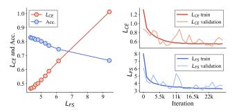
Figure 6: Correlation between  $L_{FS}$ ,  $L_{CE}$ , classification accuracy, and training iteration of the pseudo depth model. Left:  $L_{CE}$  and Acc. vs.  $L_{FS}$ . Right:  $L_{CE}$  vs. iteration and  $L_{FS}$  vs. iteration.
