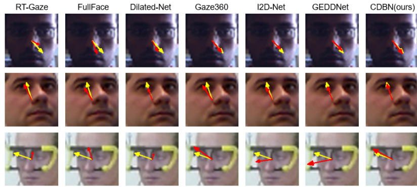
Fig. 5. Comparison of predicted gaze directions for the input size of 32 \times 32 . Three examples, one from each dataset, are included. The yellow arrow indicates the ground truth gaze and the red arrow indicates the estimated gaze.
