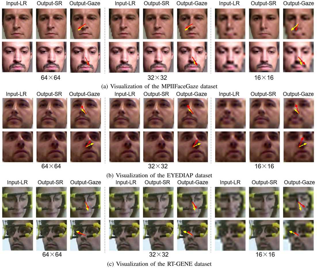
Fig. 4. Visualization of the input and output of CDBN on the three employed datasets. For each specific input resolution, the leftmost image is the LR input, the middle image is the reconstructed SR image, and the rightmost image shows the predicted gaze drawn on the LR input. The yellow arrow indicates the ground truth gaze and the red arrow indicates the estimated gaze. All images are resized to 128 \times 128 for display.
