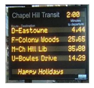
The most expensive but effective idea was placing an electronic sign at every bus stop. It would display the real-time information for every route servicing the stops. Customers would be able to view real-time information for upcoming buses and would not have to use their personal devices to check when their bus is coming.
