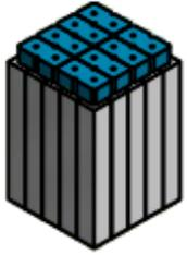
CsI[Na], deployed → decommissioned: 14.5 kg crystal, single PMT readout, LY of 13.4 PE/keV,  $\sim 8 \text{ keV}_{\text{nr}}$  threshold
