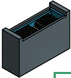
NaI[Tl]: segmented 185 kg, deployed → 2T,  $\sim 13 \text{ keV}_{\text{nr}}$  threshold (Na recoils)
