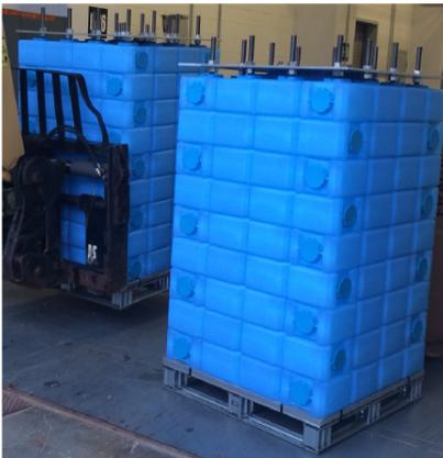
“NIN cubes” – liquid scintillator cells with Pb/Cu/Fe “shield” surrounded by multiple water modules
