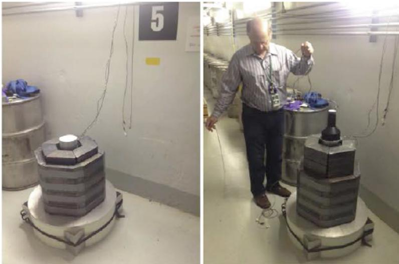
Liquid Scintillator detectors inside Lead, Poly, Cd, Water shield with muon veto
