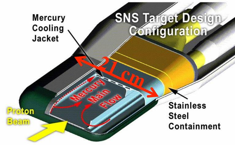
Number of protons on target for 1.1 mA at 1.3 GeV is  $0.687 \cdot 10^{16} \text{ sec}^{-1}$
