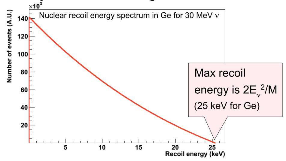
→ but WIMP dark matter detectors developed over the last ~decade are sensitive to ~ keV to 10's of keV recoils
