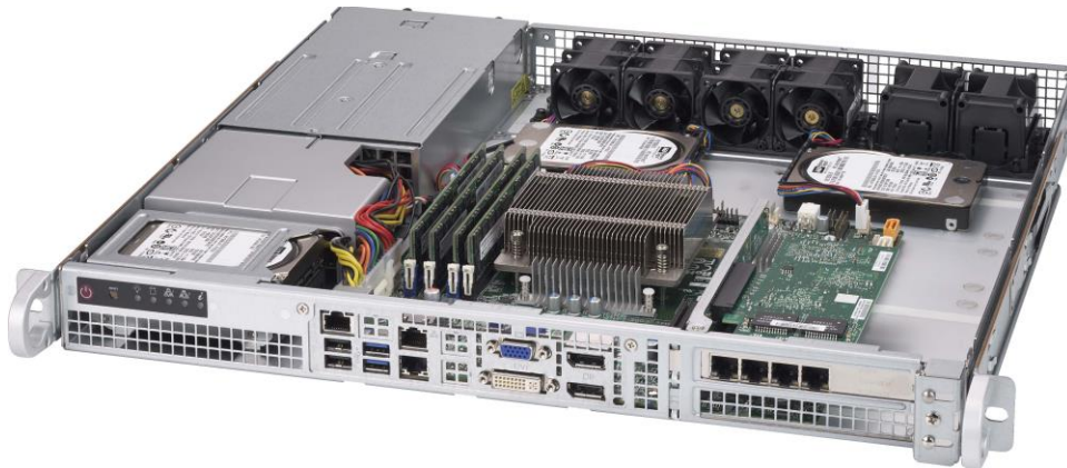
Figure 4.1 - Second Generation Appliance Chassis – Supermicro SuperChassis 515-R407
