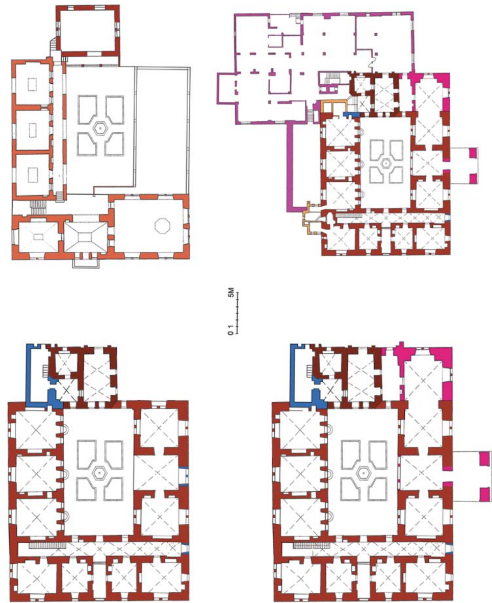
FIG. 15 Jerusalem, Rabbah Effendi al-Husseini House/American Colony: rough sketch suggesting construction phases: A. Phases I and IIA; B. IIB and IIC; C. III; D. IV and V [D. is not in scale] (drawing by A. Wharton, 2010).
