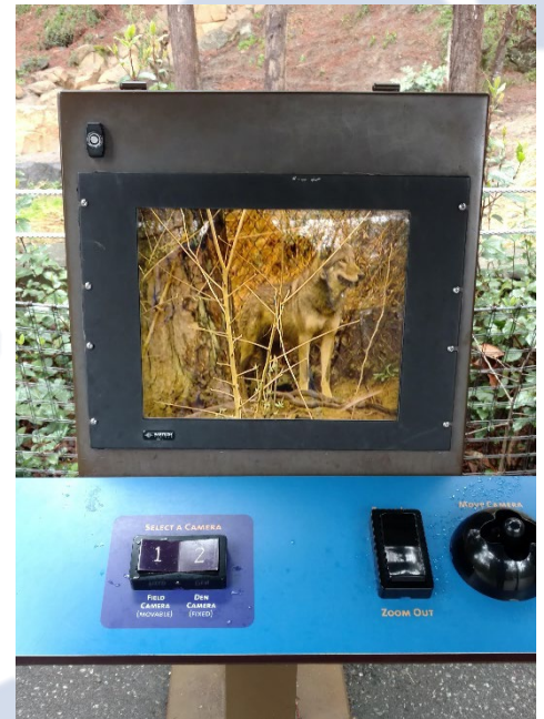
Figure 2. Exhibit camera that can be used to zoom in and track the wolves. Popular form of visitor engagement. Photo by Andrea Kolarova
