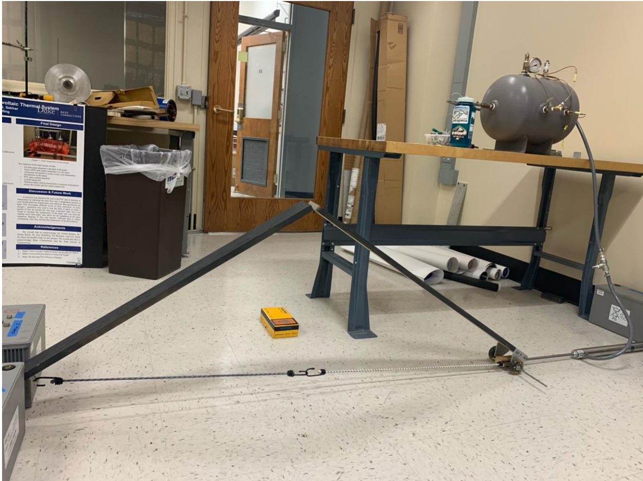
Figure 3: Rudimentary pumping mechanism
