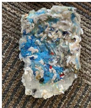
Figure 13. Brick 2 After 3-Point-Bend Test
