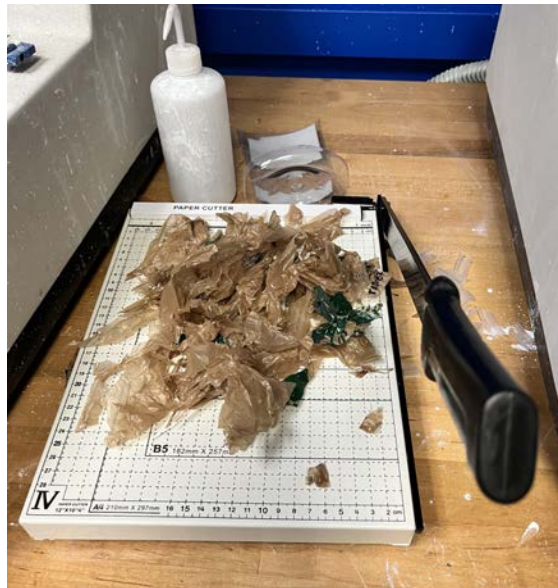
Figure 8. Guillotine Paper Cutter Effectively Shredding #4 Plastic Bags
