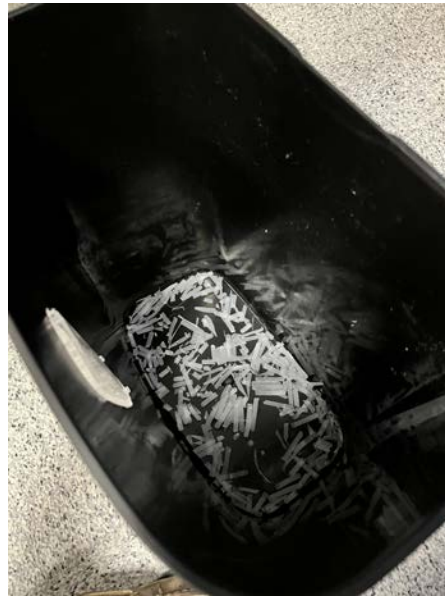
Figure 5. Plastic #2 Shredded Using the Credit Card Shredder
