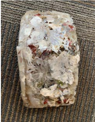
Figure 15. Brick 4 After 3-Point-Bend Test
