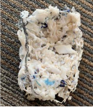
Figure 14. Brick 3 After 3-Point-Bend Test
