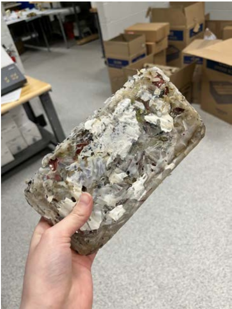
Figure 10. Completed Final Prototype for Recycled Plastic Brick (Brick 4)
