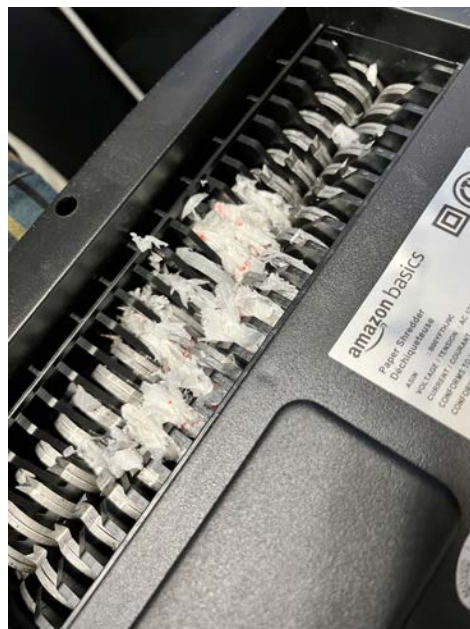
Figure 6. Plastic #4 Bags Tangled in the Credit Card Shredder
