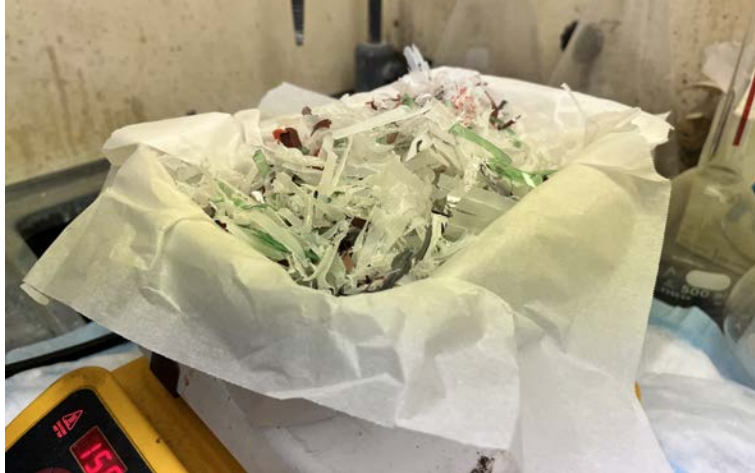
Figure 7. Medium Fidelity Process of Melting Larger Plastic Bricks with a Hotplate
