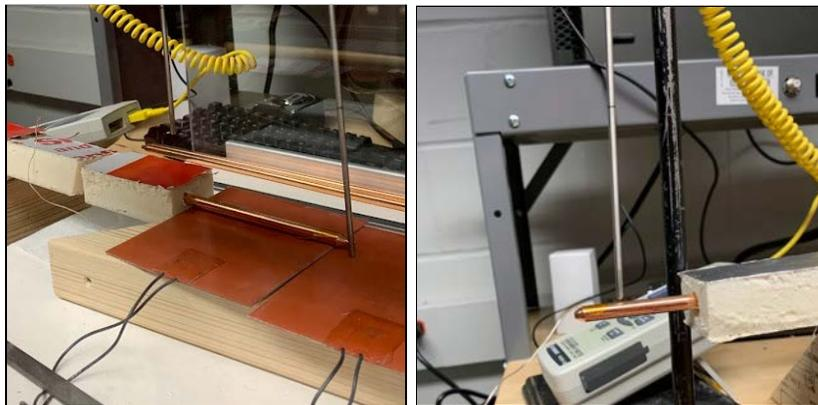
Figure 4. Thermocouples Positioned at Heat Source (Heating Pad) and Heat Sink (Ambient Air Above Condenser Length of Heat Pipe)
