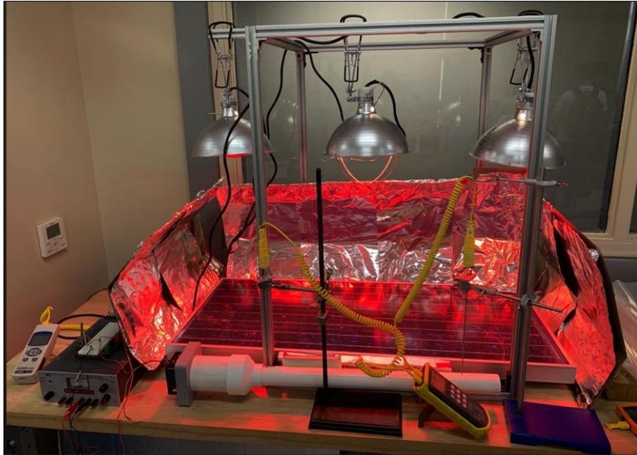
Figure 12: Final Prototype with 1.5" PVC Configuration
