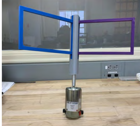
Figure 9. Kite structure model (sans fabric) attached to the motor via a 3D printed coupling.
