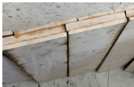
Figure 10: Photograph of the construction of a wood panel.
