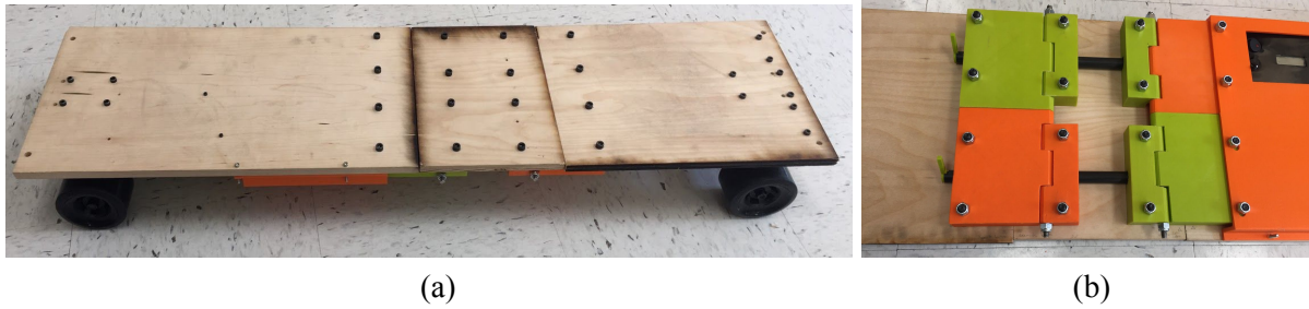
Figure 13: (a) The board in the flat and ready-to-ride position, (b) Underside view showing the structural rods in position.
