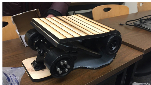
Figure 2: First prototype of a rollable design that is comprised of numerous plywood panels connected by ducktape (acting as a temporary mesh) on the underside.
