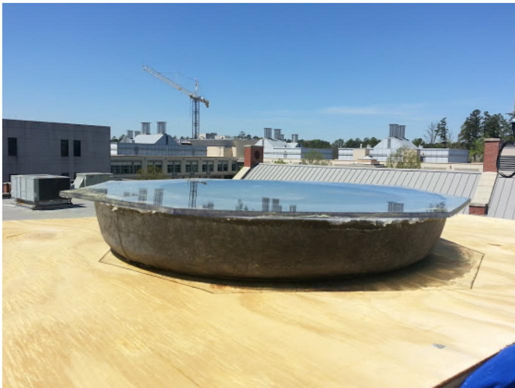
**Figure 9.1** The full-scale prototype was placed on an area of a roof that allowed undisturbed sunlight. The device was rated to hold 15-16 liters of water. To allow convenient testing,
