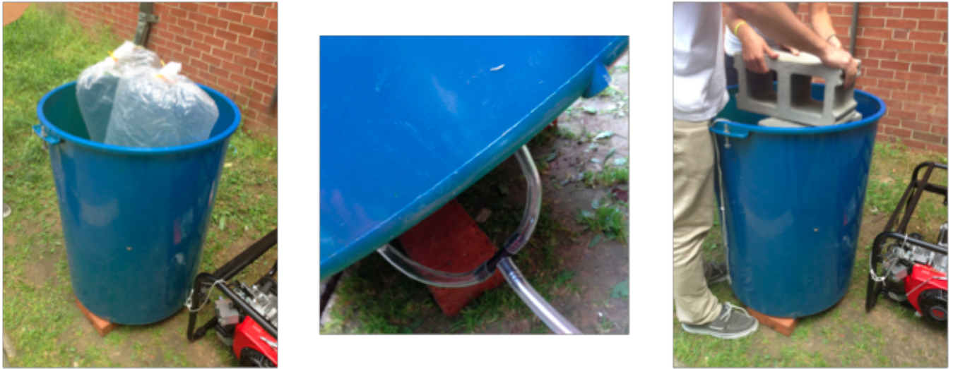
Figure 6: Plastic drum with two biogas bags, tee tube fitting, and pressurization
