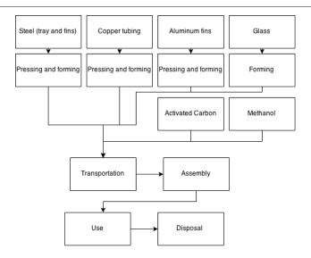
The Ecopoint 99 LCA process starts with a catalog of the materials used, the way the materials are processed, the distance and method they are transported, the amount and type of energy used to construct the product, the amount of energy used during the "use" of the product throughout its lifetime, and the energy used to dispose of the product. (See figure above.)
