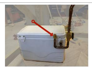
Step 2: Attach a vacuum pump to any of the three valves and draw down the pressure to less than 5 PSIA. Verify the system pressure on the gauge attached at the top of the condenser. While drawing a vacuum it may be advisable to open the system section by section.
