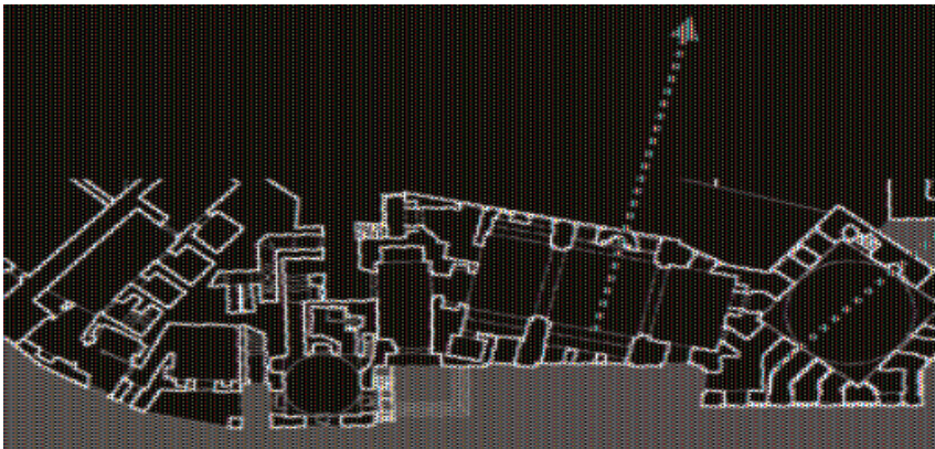
Fig. 28: Complex of Khayer Bek: Divergence between the Two Qiblas and the Varying Wall Thicknesses
